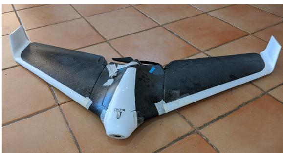
Fig. 1. The Disco Parrot UAV used to gather video data to test the proposed observer.
