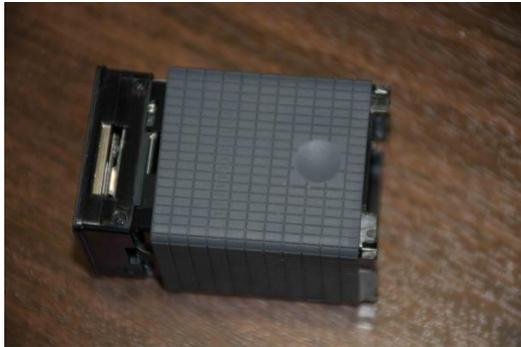
13. The rest of the screen half of the camera was pushed out of its case. This was the hardest step. Once it came out a little way, a ribbon cable was exposed just behind the screen. This cable is the only thing holding the inside and outside together. Prizing this out should allow the two parts to come apart easily. I broke this cable, although this only affected the zoom function and the camera still worked.
