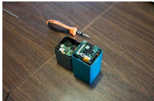
3. The two halves will not split apart, they're 4. With the ribbons remove, the pieces could still held on by 2 bits of ribbon and a plastic be slid apart. tab. The ribbons were slid out using a flat head screwdriver, allowing the two halves of the Lytro to be separated. Note that the bot- tom cable is soldered to the sensor board, and needs to be plucked off.
