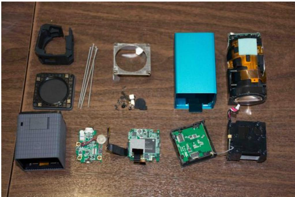
Figure A.9: The disassembled Lytro. Top row: rubber piece that attaches to outside of lens, 4 screws holding the two halves of the Lytro together, glass lens protector, cover of the lens half of the Lytro, the lens piece. Middle row: lens cover, screws, small rubber piece and small metal part attached to a screw. Bottom row: cover of bottom half of Lytro, USB board, main board with ribbon cable, battery pack with LCD screen and board attached.
