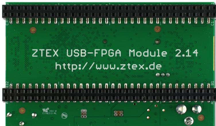
Figure G.2: ZTEX USB-FPGA-Module 2.14 Back View [8].
