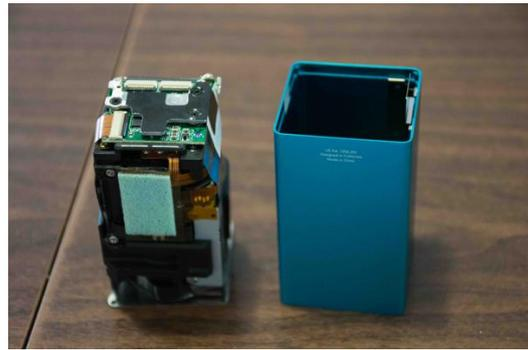
6. The lens was slid out of its casing.
