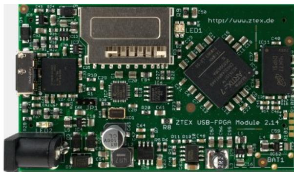
Figure 4.8: ZTEX USB-FPGA-Module 2.14 [8]
