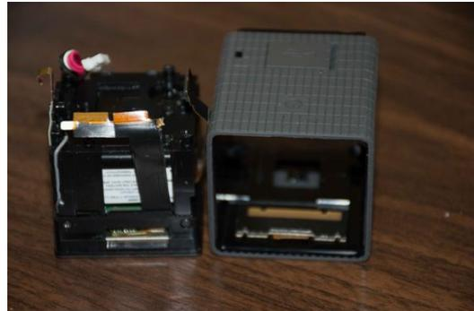
14. The LCD half of the camera removed from it's casing.
