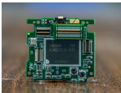
(a) Riser PCB attached to the Lytro’s main board.
