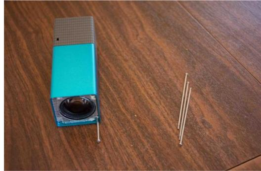
1. Heat was applied to the front of the Lytro, 2. The four long screws beneath the lens pro- loosening the adhesive tape and allowing the tector were removed. lens protector to be prised off.
