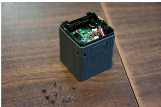
9. 8 screws and rubber cap were removed from the USB Board.
