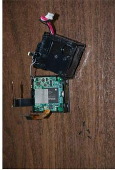
15. Unscrewing the four screws from the Main Board allowed it to be removed.
