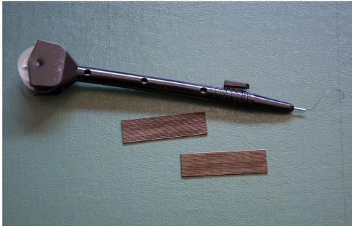
(a) Wood pieces with 0.4mm-spaced grooves
