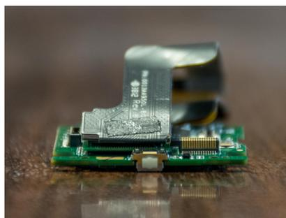
(b) Riser PCB sandwiched between the main board and ribbon cable.
