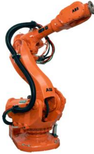
Figure 3.3: ABB IRB 6600 175/2.55 robotic manipulator
