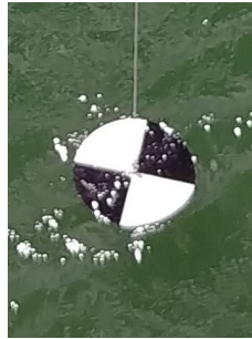
Figure 5.10: The black and white SD is being lowered into the water at Port Adelaide River to measure the water turbidity level in terms of SD depth.
