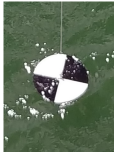
Figure 5.2: The black and white SD used for imaging.
