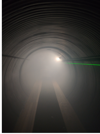
Figure 1.1: A long tunnel filled with fog. The fluorescent light and green laser on the right illustrates how light is scattered and absorbed in the fog.
