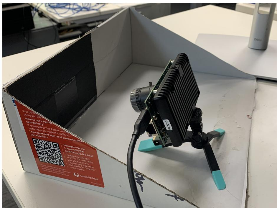
Figure A.5: Experimental setup showing the placement of the RDK within the stage during the ROI experiments
