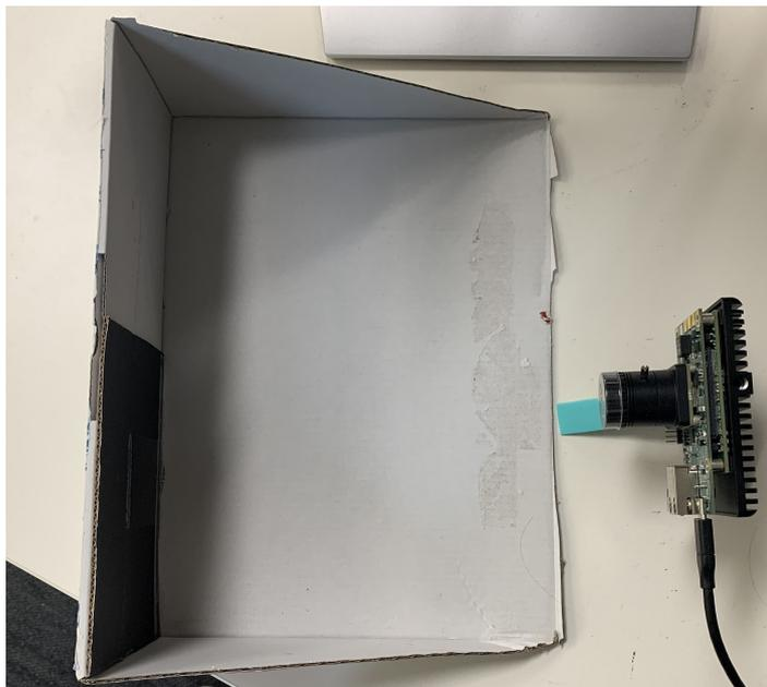
Figure A.4: Experimental setup showing the placement of the RDK within the stage during the polarity experiment
